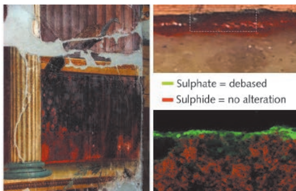
Figure 1.5.14: A wall showing the severe damage due to blackening of cinnabar in Poppea's villa in Oplanti (left). Visible light microscopy image showing debased and intact layers (pigment) and limestone (substrate) (top right). \mu XANES allows the identification of the debased layer (bottom right).
