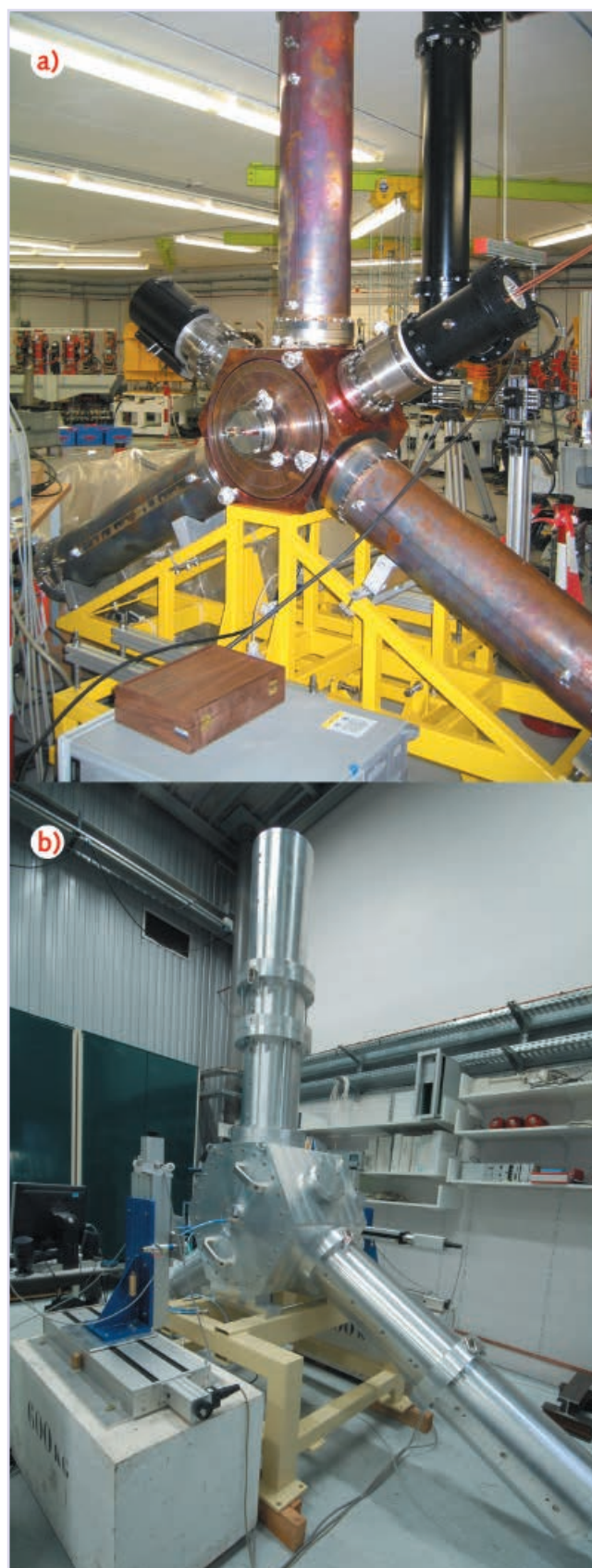
Figure 3.1.11: Normal conducting cavity with three attached ridge waveguides and ferrite absorbers for efficient HOM damping. The ESRF is actively engaged in collaborating with BESSY and ALBA to develop such a cavity for the ESRF Upgrade. a) 500 MHz HOM damped cavity on the Willy Wien Metrology Light Source. b) 352 MHz aluminium prototype in the ESRF RF laboratory.
