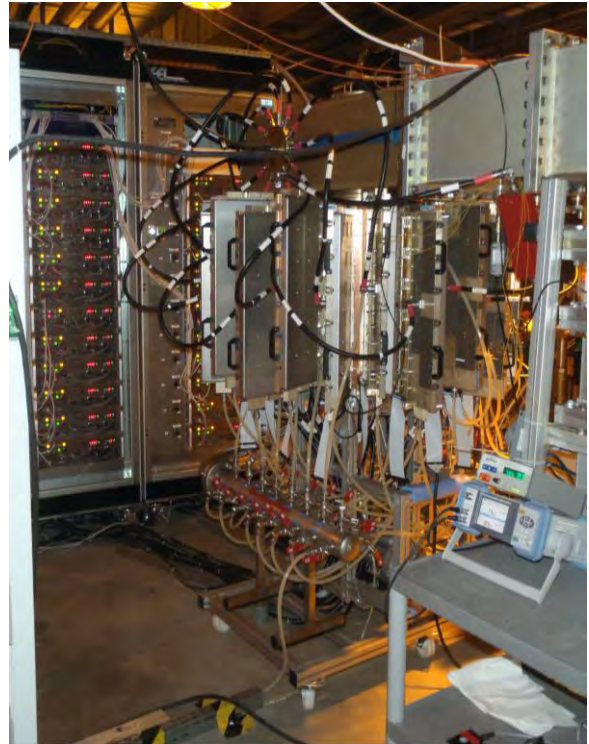
Figure 5.16: In-house 85 kW SSA. Left: during assembly in the lab. Right: during power tests.
