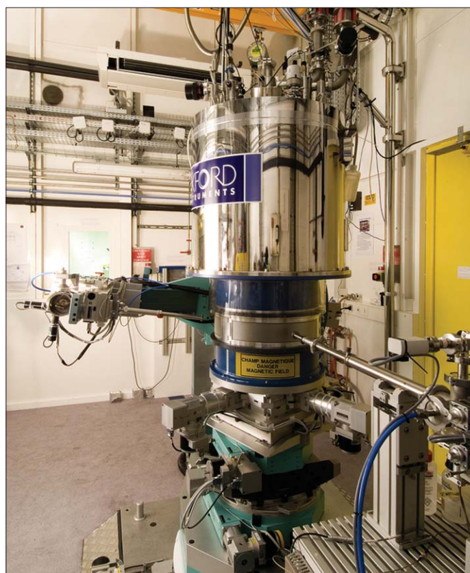
Figure 1. Superconducting 10T split-pair magnet (Oxford Instruments) on the a-magnetic six-circle diffractometer (Huber GmbH) in the ID20 second experimental hutch.
