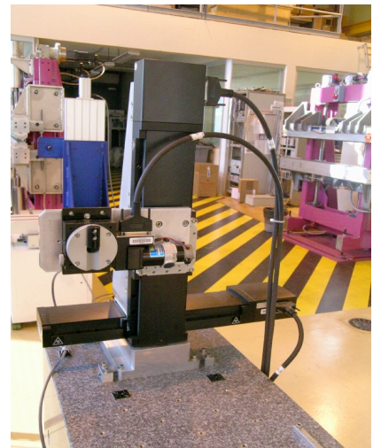
Figure 2: View of a motorized assembly of a flip coil bench
