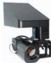
KiloRAD PTZ radiation resistant camera with Pan/Tilt/Zoom
