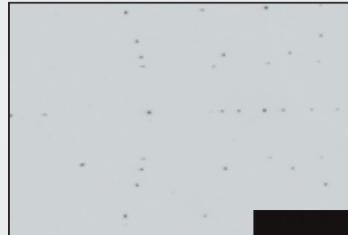
colloidal goethite nanorods 50 \mu beam size, bending magnet BM26 @ ESRF
