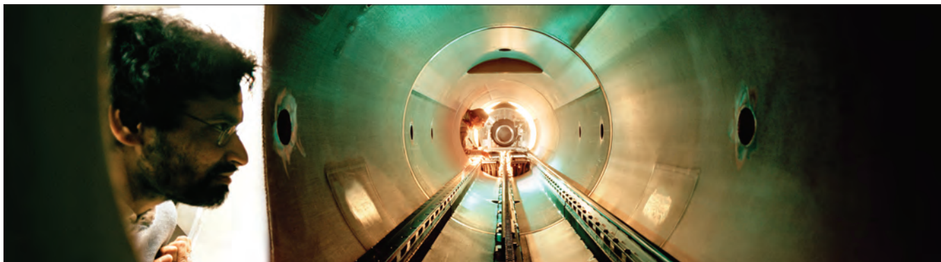
Change ahead: a movable detector for small-angle scattering studies on the ESRF's ID02 beamline.
