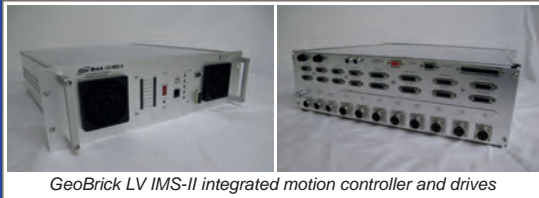
GeoBrick LV IMS-II integrated motion controller and drives
