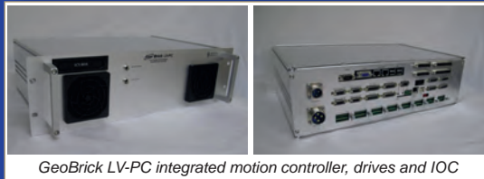
GeoBrick LV-PC integrated motion controller, drives and IOC
