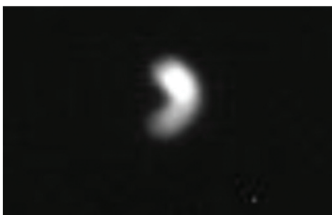
Beam spot from X-ray multilayer optic "FOX3D" of lab source into unfocused plane at 8keV and 4.108ph/sec
