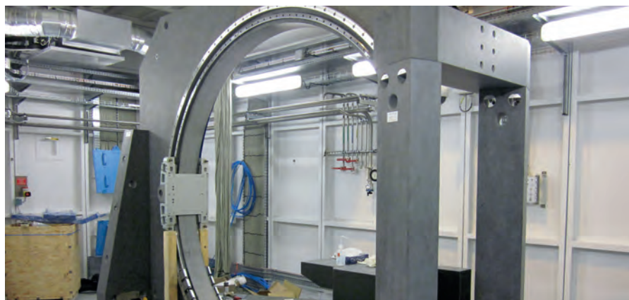
The 3 m wide, 3.2 m high granite support for ID20's Raman spectrometer.
