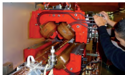
New vacuum chambers and chicane magnets were also mounted during the shutdown.
