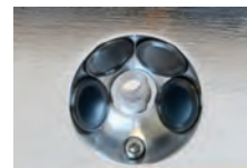
4 Sensor 'Beam Through' Detector Circular Focused Array SDD
