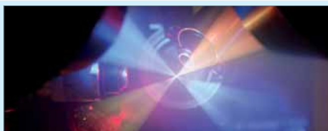
The new offline microspectrophotometer at the ID29S-Cryobench. Three LEDs (blue, green and red) have been used to visualise the intersection of the focal volumes of the three optical objectives.
