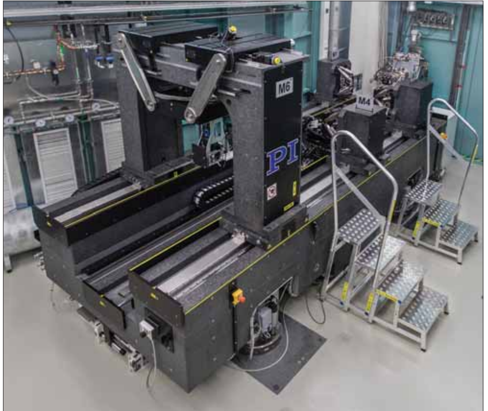
Instrument for hard X-ray microscopy and quality assurance (MiQA). PI miCos designed and manufactured MiQA and installed the machine at the IMAGE beamline at KIT.
