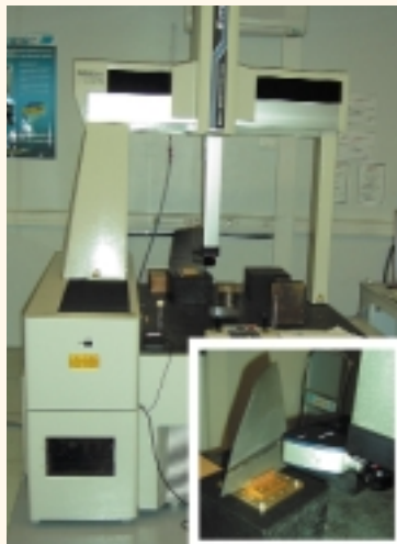
The FaME38 Coordinate Measuring Machine (CMM), which is equipped with an advanced non-contact laser metrology head (inset).
