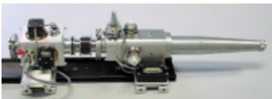
Fig. 1: The XMaS in-vacuum slit system and how it can be 'vacuum integrated' with the 'tube slits' to form a beam collimator.
