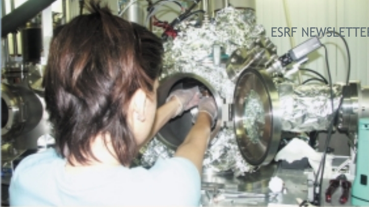
Positioning of the ceramic samples in the vacuum chamber.
