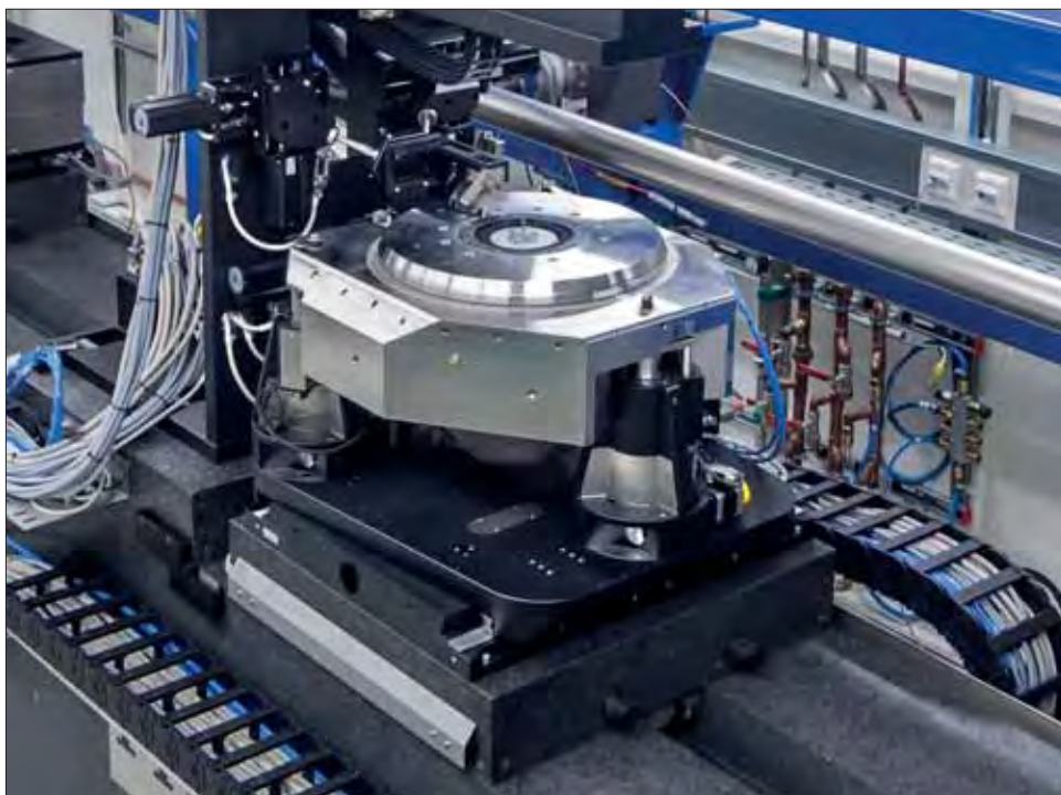
Mounted on the combined tilt and Z stage (consisting of three differentially controlled lifting elements) is an air-bearing supported rotation stage. It rotates at a velocity of up to 36°/s and works with flatness deviations of less than 100 nm at a resolution of 0.5 \mu rad (Image: PI /HZG)
