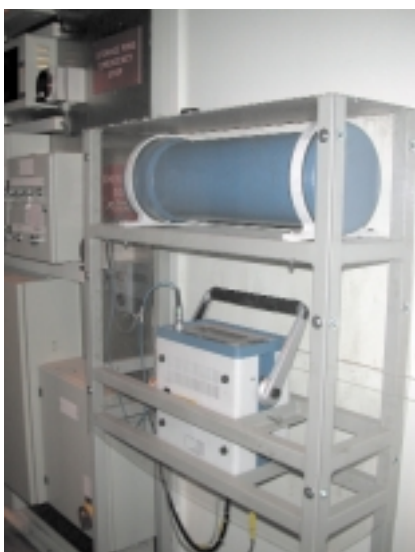
Fig. 1: Radiation monitor close to the hutch of a beamline.
