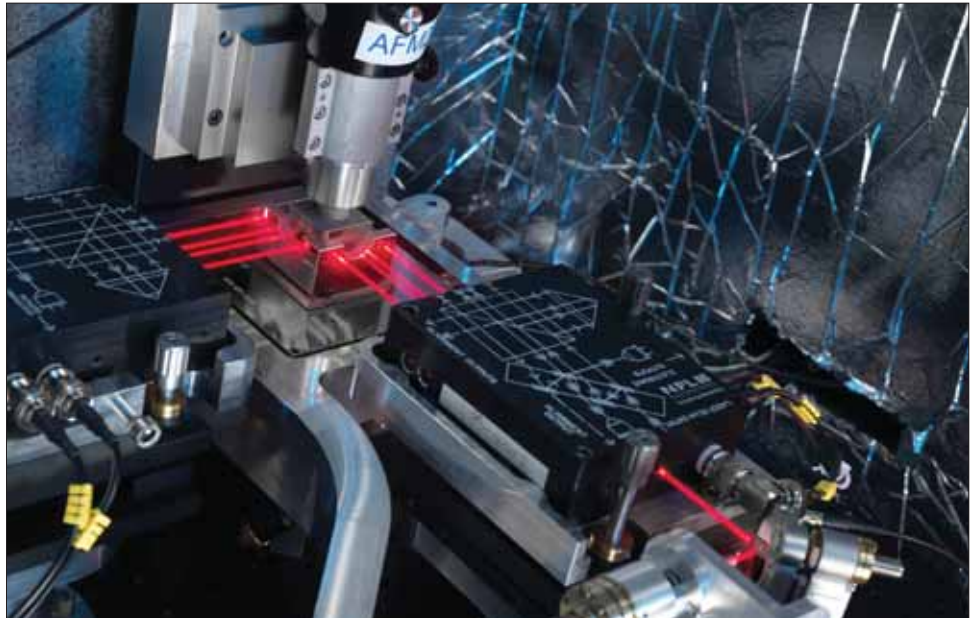
Queensgate XY stage in AFM at National Physical Laboratories.
