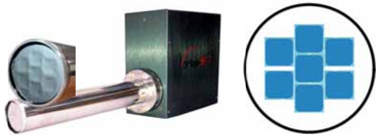
VORTEX ME-7 SDD— 38 mm diameter Detector - the same as the current VORTEX ME-4 SDD
