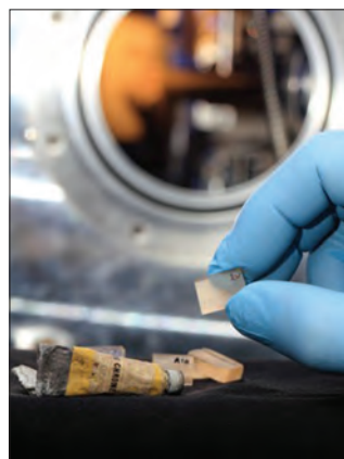
Microsamples from van Gogh masterpieces were moulded in Plexiglass and placed in the vacuum chamber of the ESRF's X-ray microscope.
