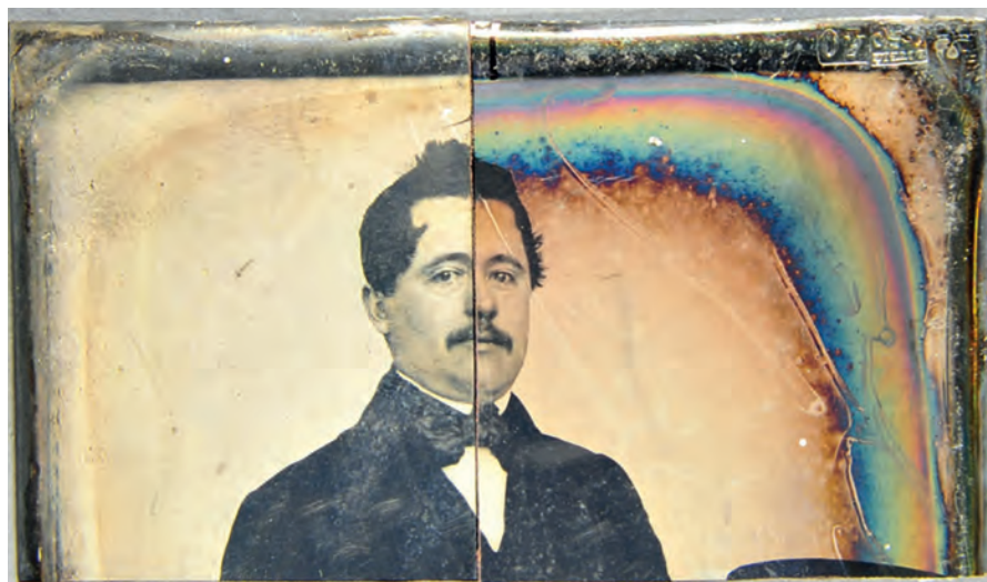
A daguerreotype photo before (right) and after (left) plasma treatment. Studies at the ESRF show that such cleaning processes are not harmful to the material's microstructure.
