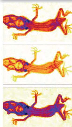
Images of a small dry animal obtained simultaneously by : a) counting the X-ray photons with a low energy threshold (LOW COUNTER, all photons); b) counting the X-ray photons with a higher threshold (HIGH COUNTER, high energy photons); c) subtracting the previous pictures one from another (low energy photons)
