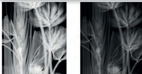
Images of a very low contrast object, taken: a) at 1 keV threshold (200 electrons, LOW counter, all photons); b) at 6 keV threshold (1200 electrons) in a single shot
