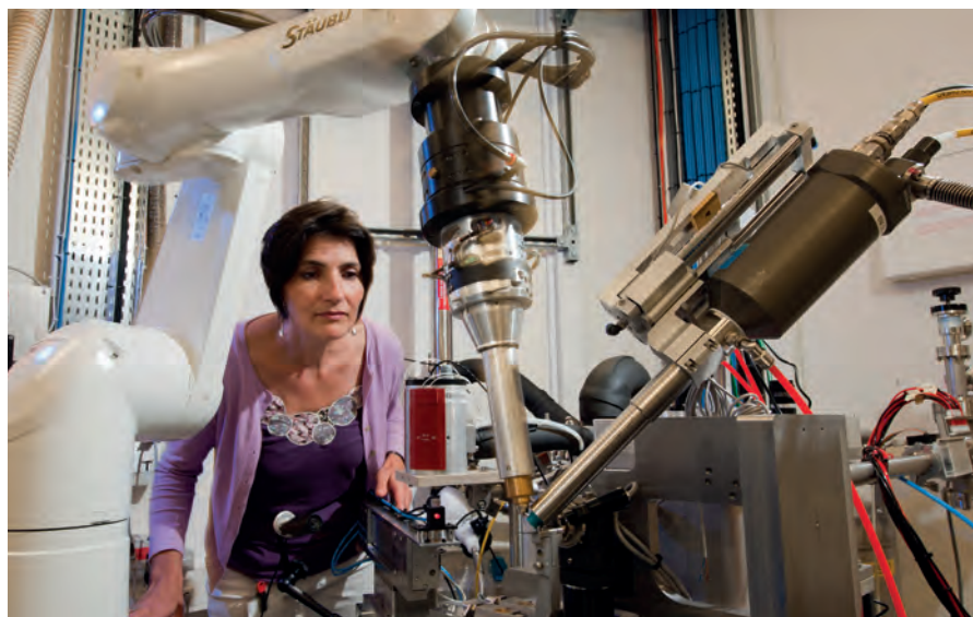
Stephanie Monaco and the robotic sample changer at the new MASSIF-1 end station.
