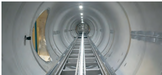
Inside view of the 34 m-long detector tube at ID02.
