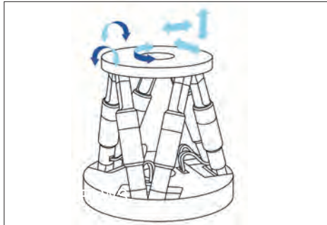
Fig 2: Basic design: In parallel-kinematic systems, all actuators act directly on the same platform. (image: PI)
