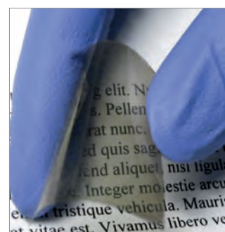
Electrically darkened material.
