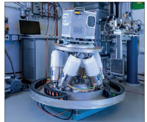
Fig 3: Hexapod in the experimentation station EH3 on the P07 beam guidance unit on PETRA III: With its high load capacity, it can carry the entire measuring setup including the structure where mechanical forces are applied – in this figure a chamber for the laser-welding of titanium aluminides. (image: PI / HZG)
