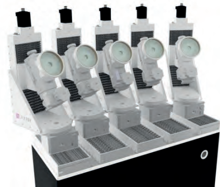
Five-crystal Johann-type x-ray emission spectrometer
