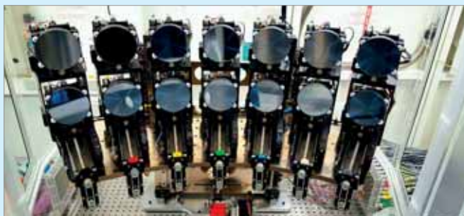
The new 14-crystal high-resolution spectrometer on BM16 (FAME-UHD).
