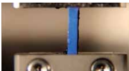
Left: In its regular state, the elastomer is light blue. Stretch it, and its colour deepens.
