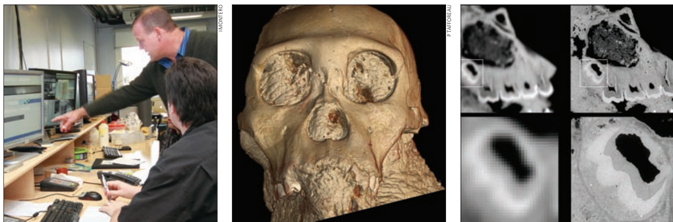
Left: Lee Berger and Paul Tafforeau discuss the data at ID17. Centre: rendering of the 3D scan of the skull of an Australopithecus sediba child. Right: comparison of a classical computer tomography scan (left) with a scan using synchrotron microtomography (right). The lower images are of a tooth. To study the development of teeth, a resolution of between 10 and 100 times higher than that used on this image is required.
