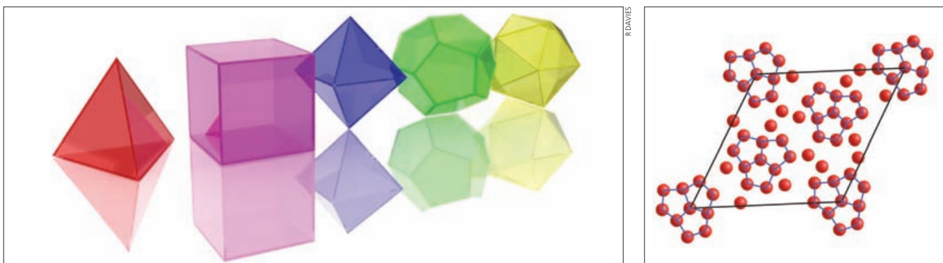
Left: the five Platonic solids: tetrahedron, hexahedron (cube), octahedron, dodecahedron and icosahedron. The first three structures are found as atomic arrangements in crystals while the latter two cannot form space-filling periodic structures due to their five-fold symmetry. The supercooled liquid droplets of this study were produced on a surface containing a large fraction of atoms arranged in pentagons (right).
