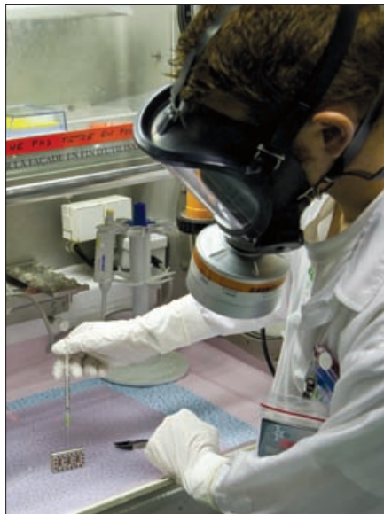
A scientist fills the inner cell with a liquid sample at the Atalante facility. Protection equipment is mandatory, including hot lab hoods and a respiratory mask.
