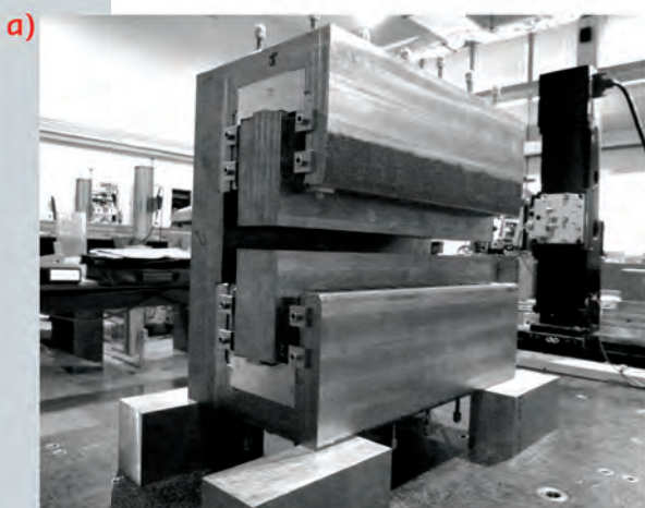
Figure 2.23: Design of electromagnet dipole with longitudinal gradient.
