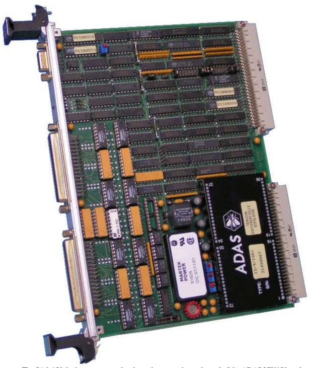
The SAdc150 device server was developped to control any channel of the ADAS ICV150 analog to digital converter board.
