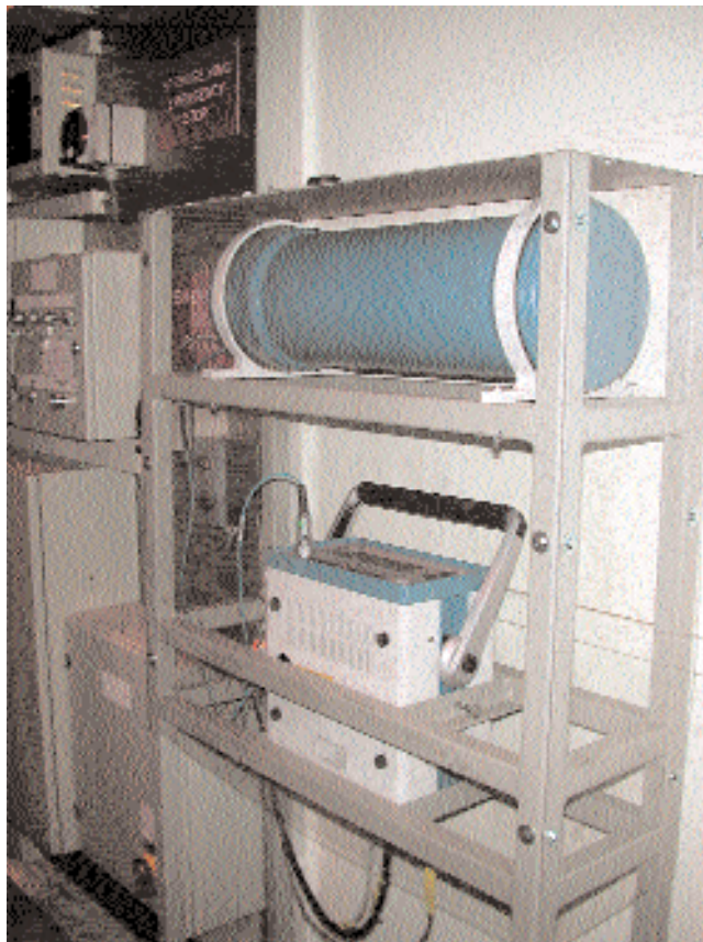
Fig. 176: Ionisation Chamber monitoring the dose rate close to the hutch of a beamline.
