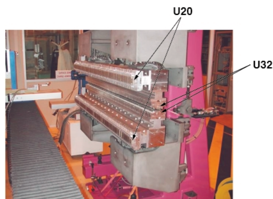
Fig. 179: Revolver support equipped with a U32 and a U20. This device is now installed on the ID18 straight section.
