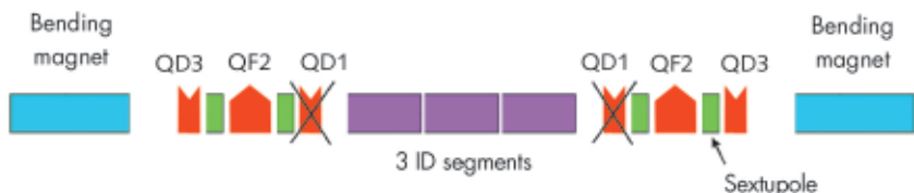
Fig. 141: Schematic lattice design of a long high beta straight section. Bending magnets, quadrupole and sextupoles are shown in blue, red and green respectively. The segments of the insertion devices are represented in purple. With the new lattice in use, the quadrupole family QD1 on both sides of the insertion devices is no longer powered and can be removed extending the total length of straight section available to insertion devices from 5 to 6 m. On the low beta straight sections, the quadrupole families QD1, QF2 and QD3 becomes QD8, QF7 and QD6. The last quadrupole QD8 adjacent to a low beta undulator have been switched off in the new lattice settings.
