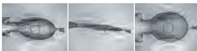
Fig. 160: (top) Examples of the composite images built from visible light images taken at different focal lengths to overcome depth-of-field issues; (lower) The three-dimensional model of the insulin crystal, buffer and loop built from the images. Blue shows the crystal and loop components, and red the cryocooled buffer. The circle on the lower image shows where minor errors are apparent in the model.
