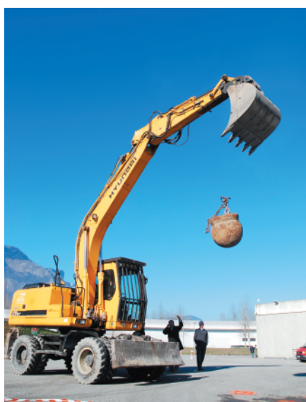
Fig. 4: Vibrating the floor of the ESRF (February, 2008).
