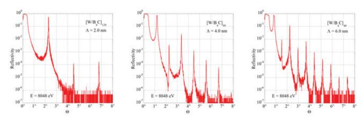
X-ray reflectivity data at E = 8048 eV of W/B<sub>4</sub>C MLs with d-spacings of  $\Lambda$  = 2.0, 4.0, and 6.0 nm. High reflectivity and visibility of higher reflection orders indicate ordered stacking and sharp interfaces.
