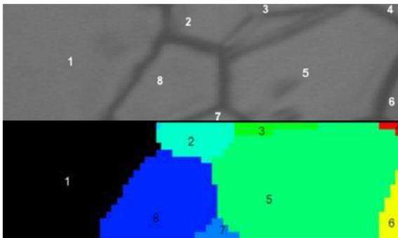
Fig 2: Comparison between our microscope image and grain size and orientation as determine by the white beam raster scan on a UO2 sample. A perfect correlation is clearly visible.
