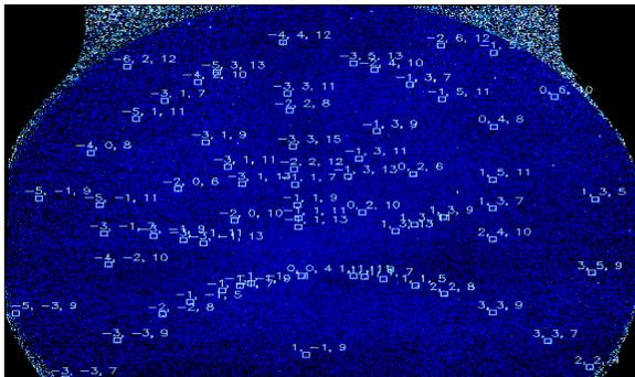
Fig 1: 0.15s recorded Laue diagram of a reference Si(001) wafer. More than 50 Laue diffraction peaks are visible and were indexed.
