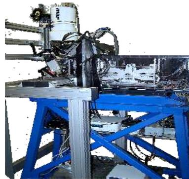
Fig 3: picture of the microdiffraction setup on its dedicated support in blue (cross reinforcement bars are clearly visible). KB mirrors are inside a transparent N2-filled chamber. On the top left, the MAR CCD camera is visible and at 40° our microscope.
