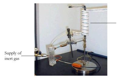
Line Drier wrapped a in Heating Tape
