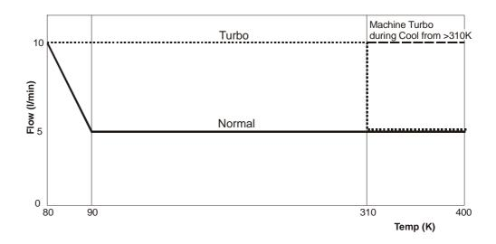
In addition to the Normal and Turbo settings, Cryostream enforces a 'Machine Turbo' during COOL phases. This corresponds to a flow rate of 10 l/min and is indicated by a flashing TURBO lamp.
